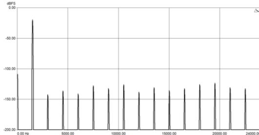
Figure 7: spectrum of 16bits, 0dBFS, 1.5kHz sine wave sampled at 48kHz, attenuated by 20dB using the alternative approach and quantized to 20 bits
