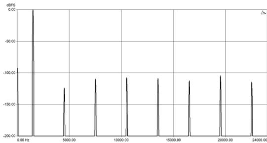
Figure 3: spectrum of 16bits, 0dBFS, 1.5kHz sine wave sampled at 48kHz
