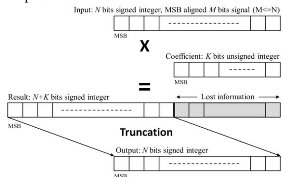
Figure 1. Digital domain volume control principle
