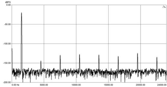
Figure 4: spectrum of 16bits, 0dBFS, 1.5kHz sine wave sampled at 48kHz, attenuated by 20dB using:
