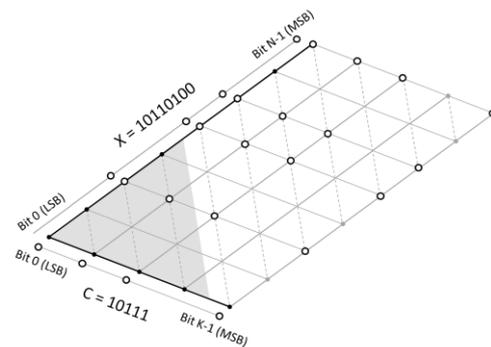
Figure 5: 2D representation of  $N \times K$  bits multiplication ( $N = 8, K = 5$ )
